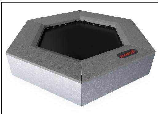
All steel components are manufactured from carbon steel S235 in a thickness of 3 mm. Side panels, support walls for top frame, plates bended with SBR and plates flat for in-situ surfacing are hot dip galvanized.
